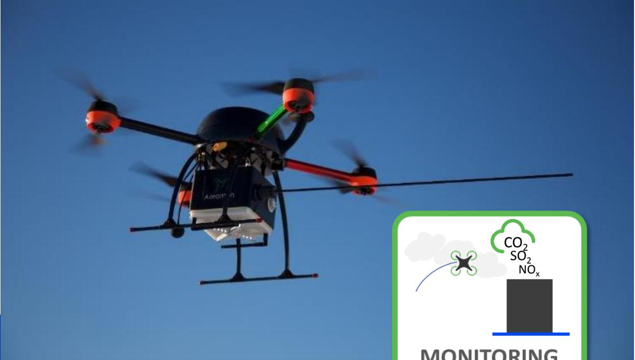
“This project demonstrates the applicability of the ultra light Aeromon BH-8 sensor module and the real time reporting tool, Aeromon Cloud service in emission monitoring.”
