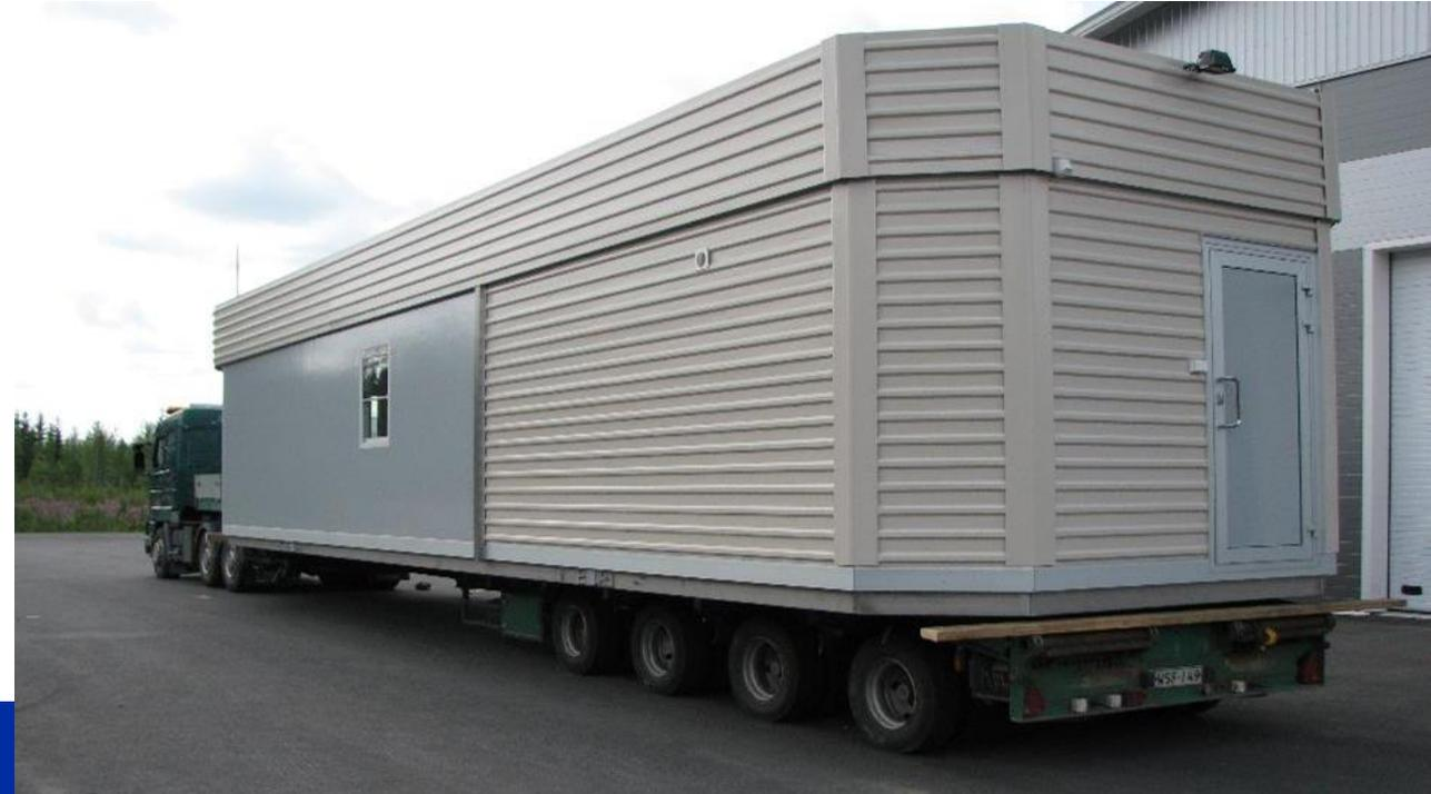
“Teles project made it possible for us. Now we can manufacture prefabricated building blocks up to 100 square meters and transport them without damages everywhere in Nordic countries. Everything is ready for “take off”. Also interior decoration if needed. Buildings were tested in Lapland in co-operation with VTT Expert Services Ltd.
