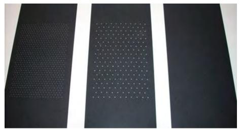
Termal absorber plates for an unglazed thermal collector prototype
