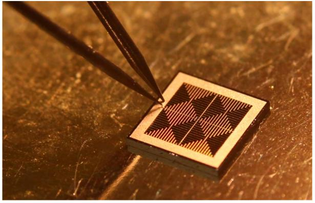
Processed III-V solar cell under test
